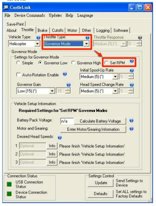
After selecting "Set RPM," you will be prompted to enter other necessary settings, such as battery voltage, Gearing Information. Should these parameters need to be adjusted in the future, click on "Calculate Battery Voltage" or "Enter Motor/Gearing Information."
